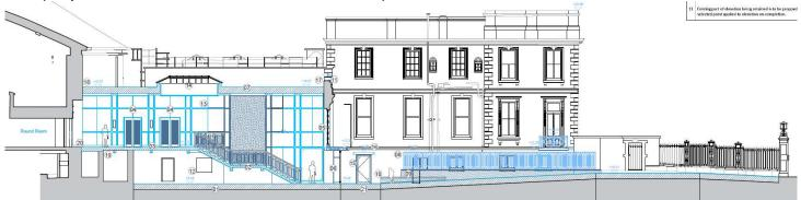
Extract from Architects' drawings of Proposed Section of New Foyer to Round Room and North Elevation of the Mansion House (Proposed alterations or additions shown in Blue)
